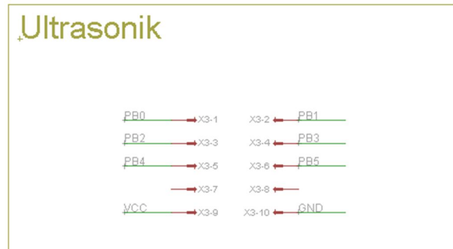
Gambar 13. Schematic header sensor ultrasonik
